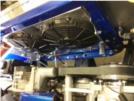
Radiator The Griffin 3 tank crossflow is perfect. It mounts in a V8 rad support and is easiest to connect to the engine. Trans cooling lines go in bottom tank. The complete kit includes condenser & dual fans.
