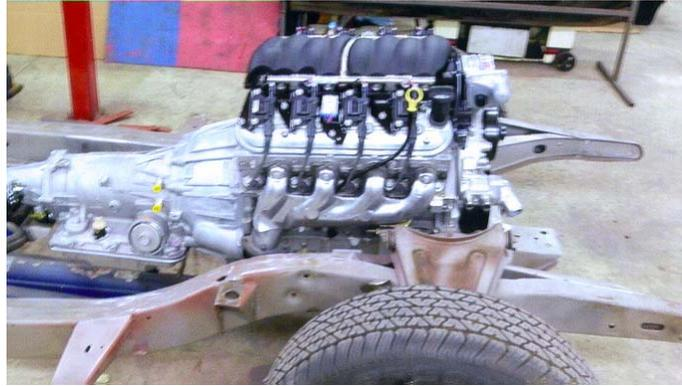
The cast iron exhaust manifolds supplied on most of the LS crate motors work perfectly and clear the power steering box we sell [#10-351]
